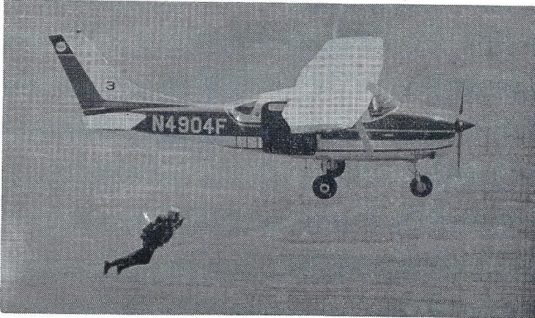
Exiting the 206 for a style jump. Note the size of that cargo door and imagine what it did to the climb rate.
