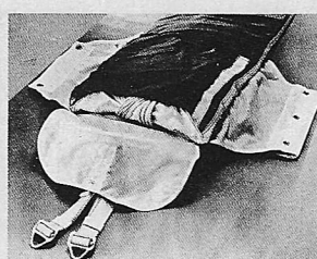
FIGURE 10 LAUNCHING SLEEVE PLACED ON PACK
