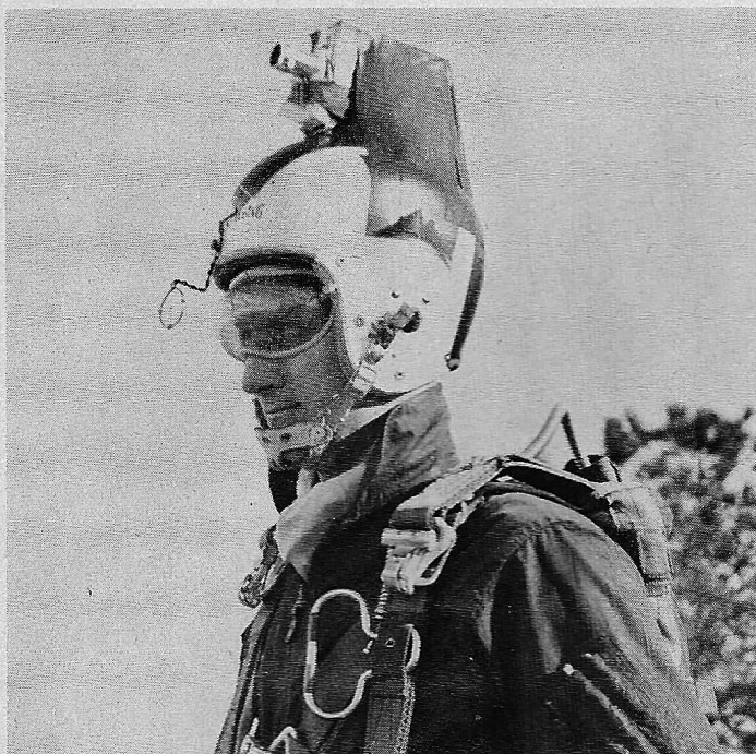
Ed Kruse Parachute Rigger 1st Class U.S.N. wears helmet and camera combination used by the Lakehurst Skydivers for mid-air photography. Note the top of helmet mounting and ring sight similar to one used by Bob Sinclair.
